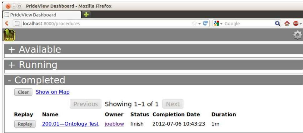
Figure 7. The PRIDE View summary screen shows the current changes to the procedure execution database that the user has made.
